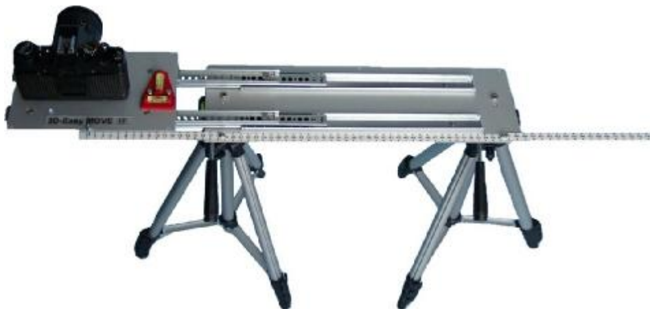
Self made special tripod to produce basic images for a 3D lenticular image
