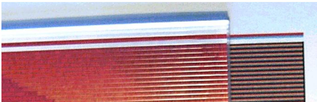
Perfect alignment: lenticular card and printed image run parallel.
