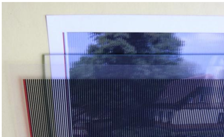
Sequence with the barrier-print: printed stripe image > glass > stripe mask
